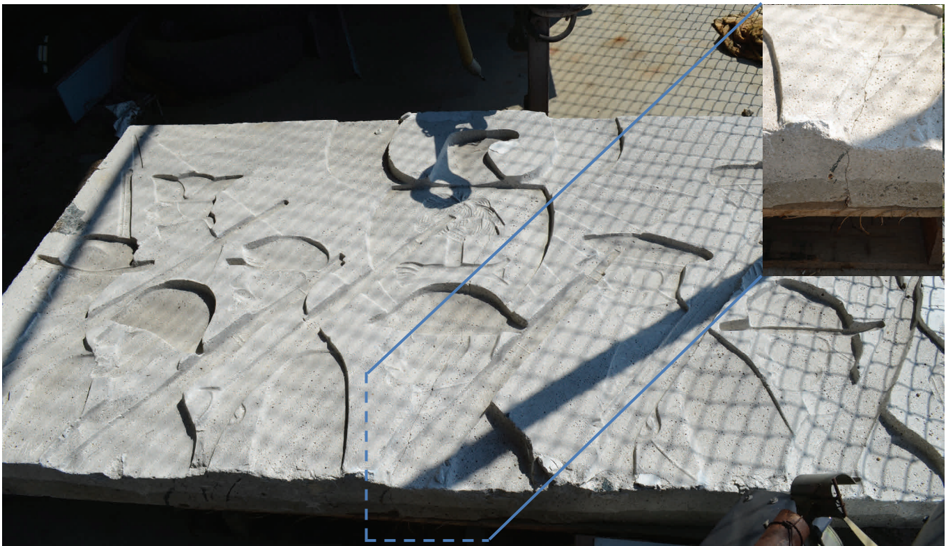
Figure 1. Hirsch panel mold at the South Carolina Military Museum. Inset image shows a major crack in mold.
